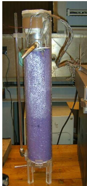
Fig.2 Storage tank full of PCM.
